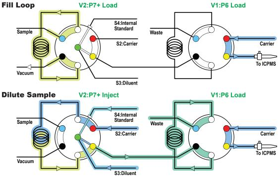
**Figure 2.** The prep*FAST* system schematic illustrating 1) sample loading during spray chamber rinse and 2) sample injection dilution and internal standardization.
