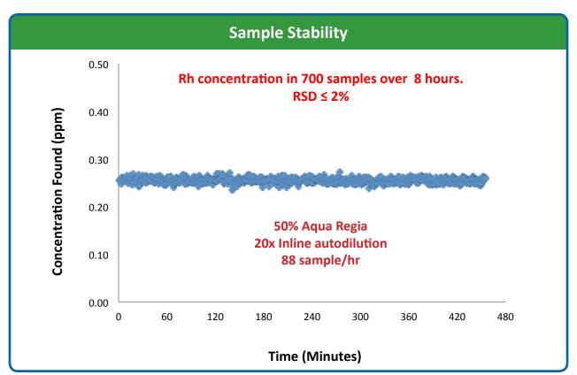
**Figure 4.** A 5ppm Au, Os, Ir, Pt, Pd, Rh, and Ru sample prepared in 50% Aqua Regia simulates a fire assay digestion. The concentrated mineral acid solution is diluted 20x inline for 700 replicate sample analysis of 0.25 ppm of precious metals. prep*FAST* inline autodilution illustrates not only a rapid throughput at 88 samples per hour, but also very accurate reproducible results for a 50% Aqua Regia matrix.
