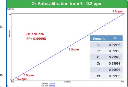
**Figure 1.** prep*FAST* automatically generates a 0.2 (25x), 0.5 (10x), 2.5 (2x) and 5.0 (1x) calibration curve from a 5 ppm Au, Ir, Os, Pd, Pt, Rh, and Ru (5% HCl/5% HNO<sub>3</sub>) stock standard solution. Precise and accurate syringe based inline autodilution is illustrated through excellent linearity of all calibration curves.
