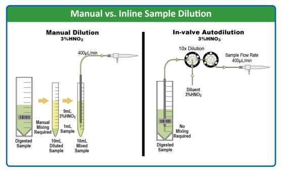
**Figure 3.** Mixing inline eliminates the need to premix/dilute samples in discrete tubes prior to analysis. This cost effective approach improves sample throughput, saves time, and reduces labware and reagent consumption. After in-valve dilution, the sample is injected (400  $\mu$ L/min) at the user's desired flow rate.
