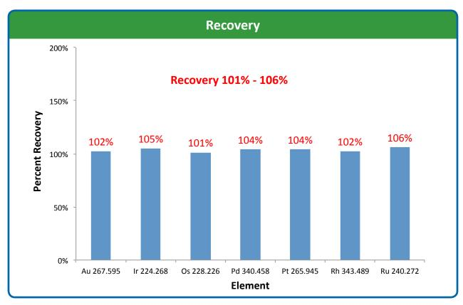
**Figure 5.** Recovery based on the 700 analysis of 0.25 ppm precious metal is both quantitative (101 to 106%) and precise (<3%).
